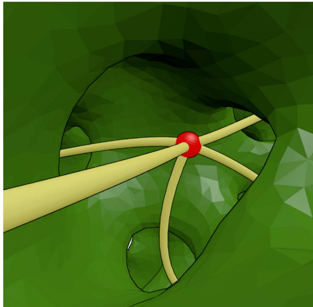
Figure 3-2: Illustration of a branch point (red dot) connecting several medial axes (yellow lines) in connecting pore channels of the carbon bijel (with its solid phase shown in green).
