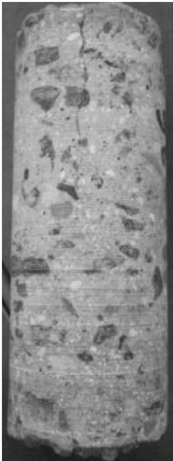
Figure 4-2. Core showing crack initiation at the surface of the slab at a Palmdale test section (photograph from Heath and Roesler, 1999).
