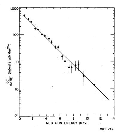
Fig. 3. A plot of  $\ln \frac{d\sigma}{d\Omega dE}/E^{5/11}$  as a function of neutron energy for the neutrons resulting from 190-Mev proton bombardment of natural uranium. The points are based on the average of the 45° and 135° data. The errors indicated are statistical errors. According to LeCouteur, 8 the data should fall on a straight line with the slope  $-11T_0/12$ , where  $T_0$  is the initial nuclear temperature. The straight line represents  $T_0 = 1.9$  Mev.
