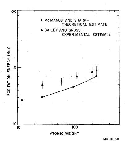
Fig. 5. The average excitation energy of the residual nucleus as a function of atomic weight of the target for 190-Mev proton bombardment.
