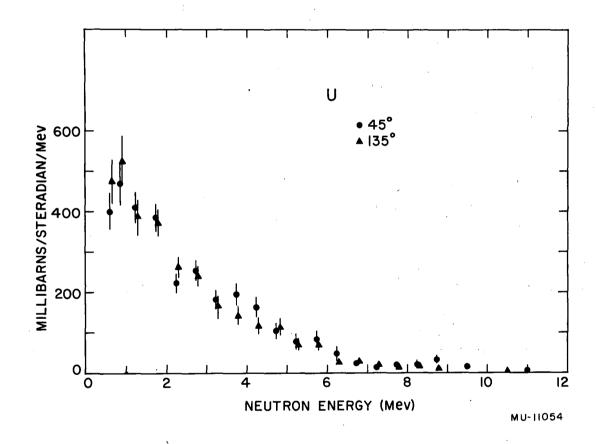
Fig. 1. Differential cross section for the production of neutrons from 190-Mev proton bombardment of uranium. The errors are statistical errors only.
