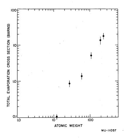
Fig. 4. Total cross section for the production of "evaporation" neutrons as a function of atomic weight of the target for 190-Mev proton bombardment.
