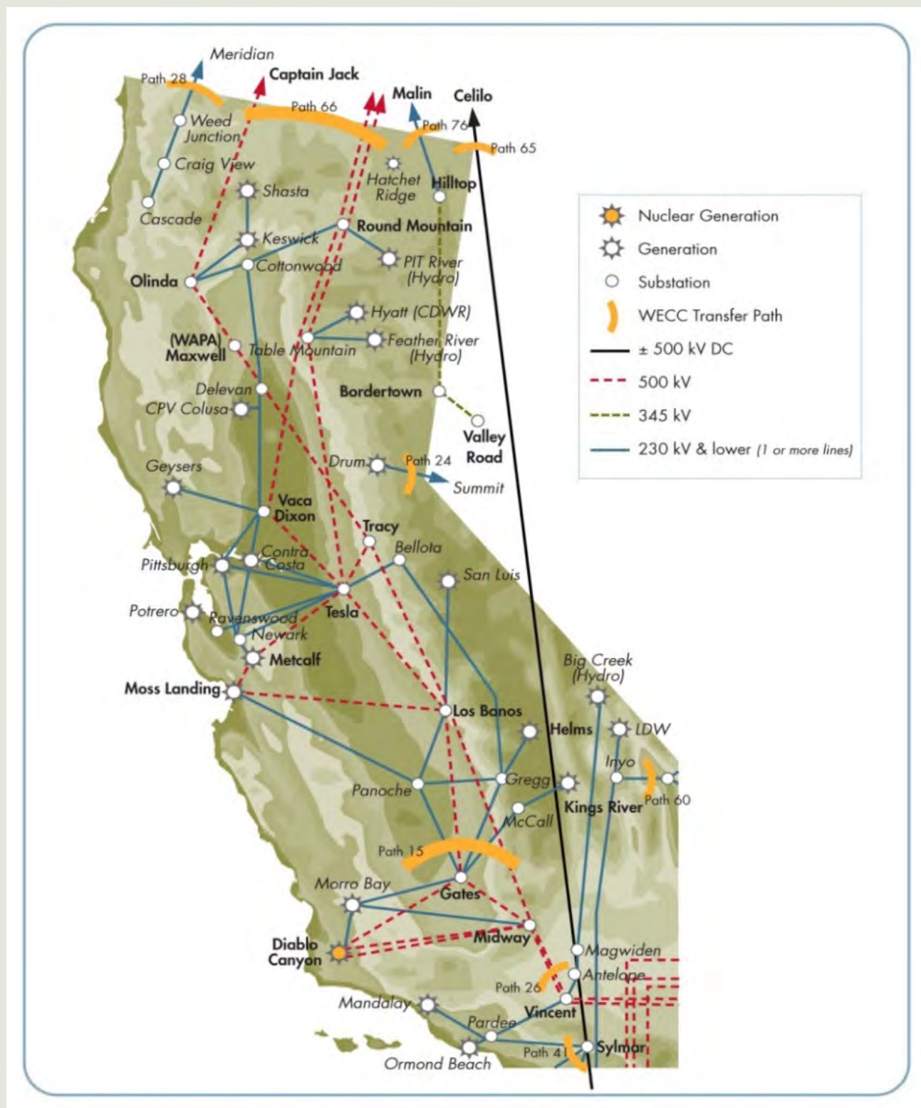
FIGURE 17. Bulk transmission system for northern California illustrating 500 kV, 230 kV, and 115 kV transmission circuits and substations within the identified boundaries of the San Joaquin Valley. The 500 kV bulk system runs along the west side of the San Joaquin boundary.
