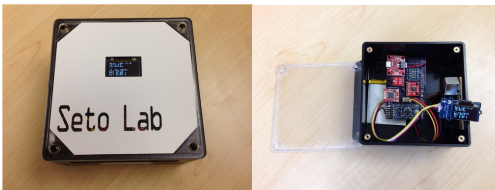
Figure 3-1 The Portable UW Particle (PUWP) monitor (left), and internal components (right)
