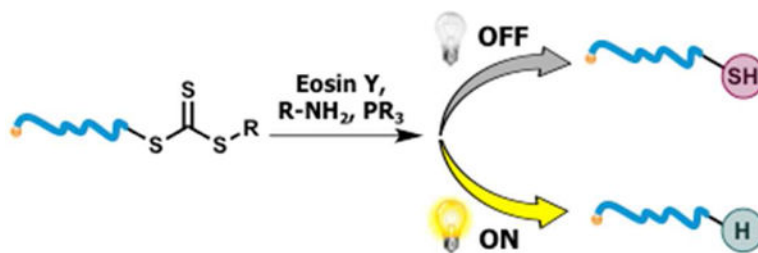
Fig. 1. Selective one-pot conversion of a trithiocarbonate CTA to either the thiol or hydrogen chain-end.
