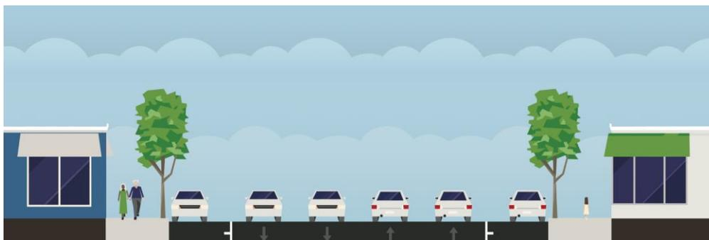
**Figure 3.** Typical Configuration After a Classic Road Diet is Implemented. *Source: Streetmix*
