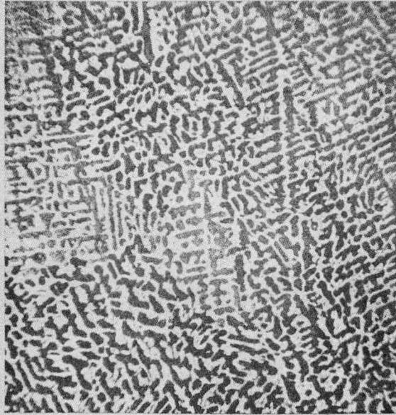
Fig. 104. Cu-Ni alloy: 50 per cent. Cu, 50 per cent. Ni. As cast. \times 100 .
