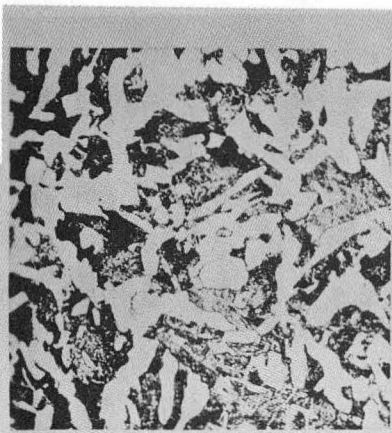
FIG. 279. Slowly cooled steel 0.43 per cent. C. \times 100 .
