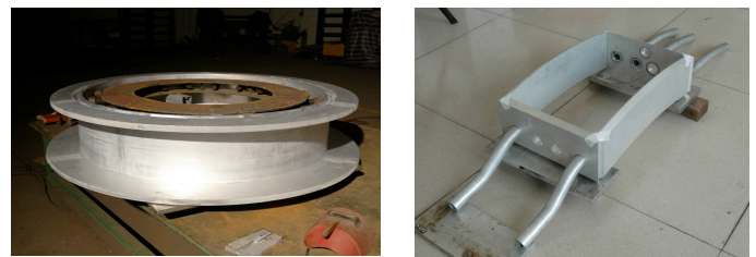
Fig.5. Mandrel after welding , pre-assembly of cooling tubing and He vessel
