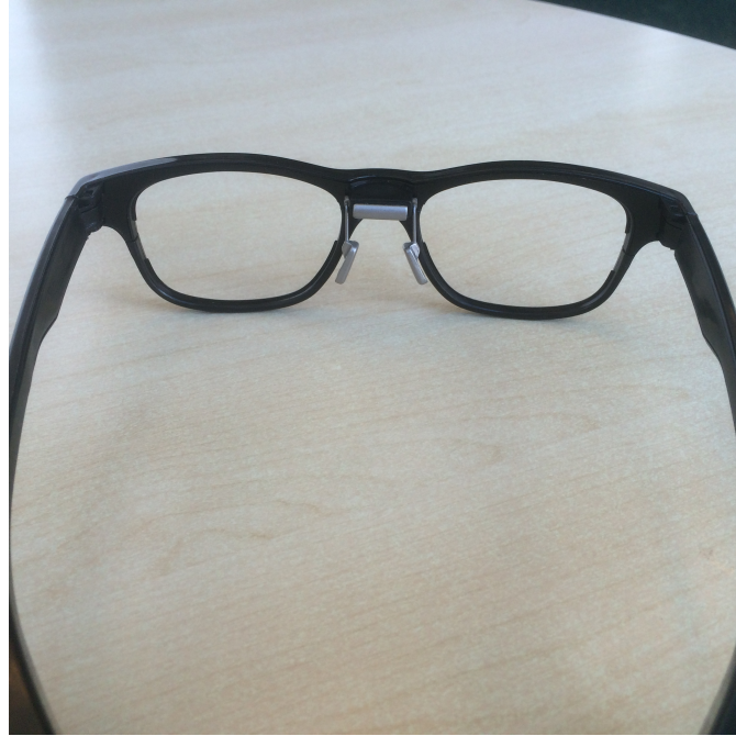
Figure 3.3. Electrode placement on the Jins Meme Glasses. The nose bridge serves as the ground reference node and the two nose pads act as the actual voltage reading nodes.
