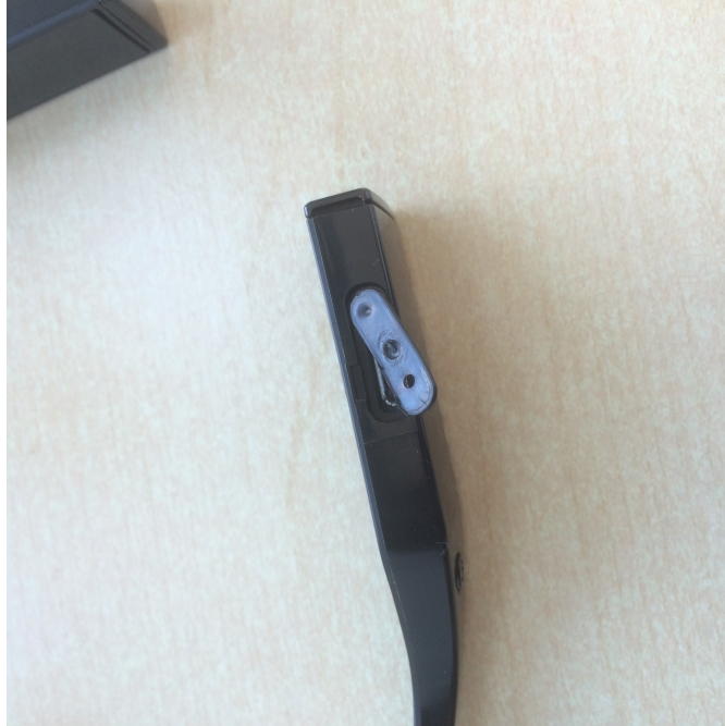
Figure 3.4. Wear and tear on the USB cover of the Jins Meme glasses.
