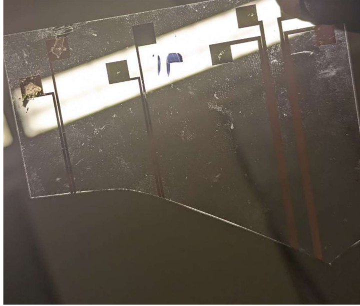
Figure 3.12: Sample 1L after all thermal cycling tests. The large damaged sections of copper are visible on traces 1 and 2 to the left. Traces 3 and 4, as well as all of the control traces, had small but visible gaps in the test pads compared to before any tests as seen in figure 2.1.
