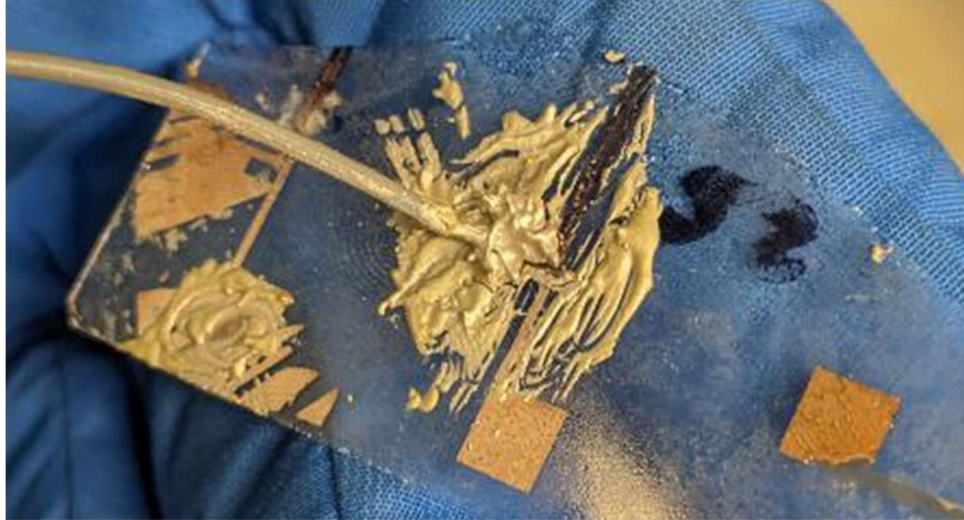
Figure 3.3: Sample 2S after the attachment of the 16 gauge copper wire using silver epoxy after one liquid nitrogen dunk cycle. Note the epoxy with no attached wires or leads on the bottom-leftmost test pad.
