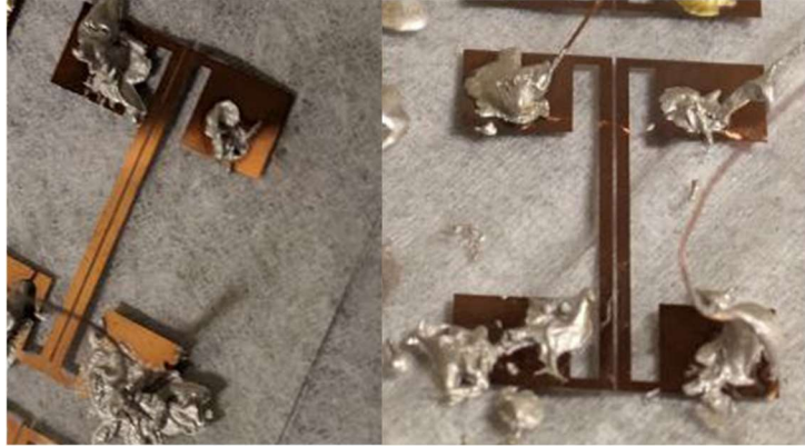
Figure 3.4: Pair 14 (left) and pair 34 (right) on sample 3. Note the lack of attached leads on the top two test pads of pair 14 and the bottom test pad of trace 34L.
