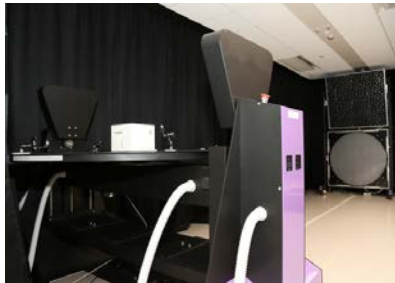
Figure 5. The heliodon component: sun simulator and turntable
