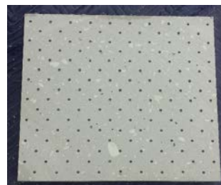
Figure 4: Translucent concret panels made with white ultra-lightweight cement composite
