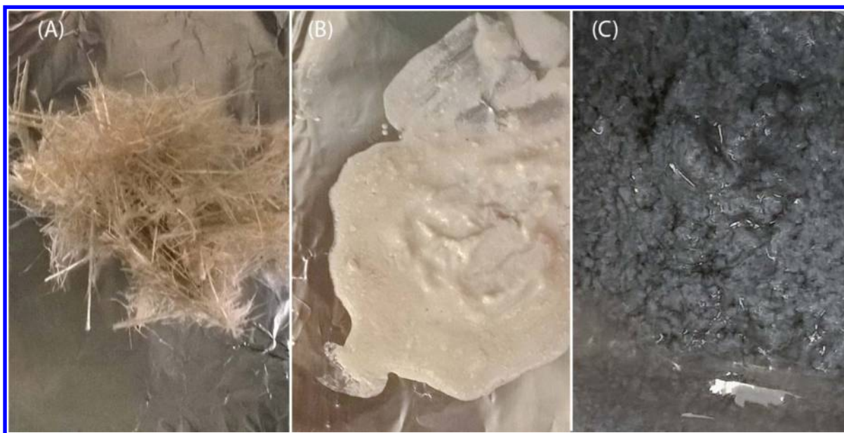
Figure 1. Grinding of chrysotile fiber bundles (A) with or without water affected the color of fibers produced. Dry grinding produced typical white fibers (B), whereas wet grinding produced gray fibers (C). The dry-ground fibers were soaked in water before the picture was taken.
