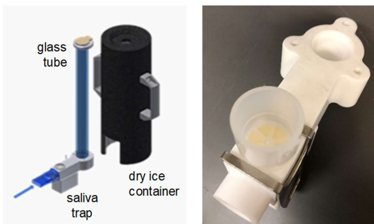
Figure 1. Description of the K-tube device (left) and the mouthpiece with the trap structure (right)
