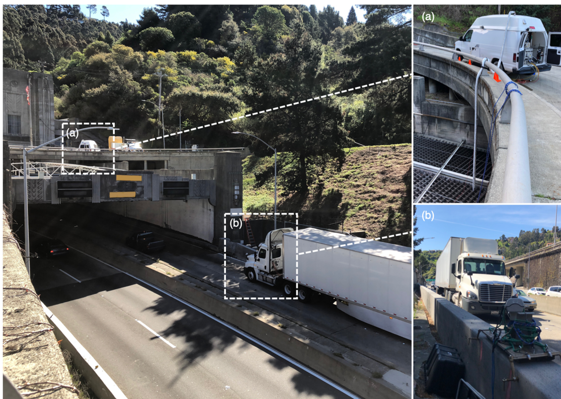
Figure 1. Field sampling site at the west entrance of the Caldecott Tunnel. (a) Pollutant concentrations were measured using a research van that was parked on an overpass above the highway, via a sampling line that aligned with the vertical exhaust stacks of heavy-duty diesel trucks passing by below. (b) A video camera next to the roadway recorded truck passing times and license plates.
