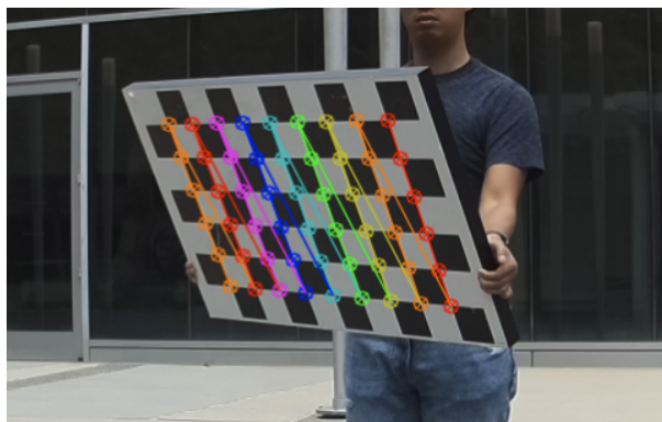
Figure 2.8. Example of calibration process, specifically checkerboard detection algorithm using OpenCV.
