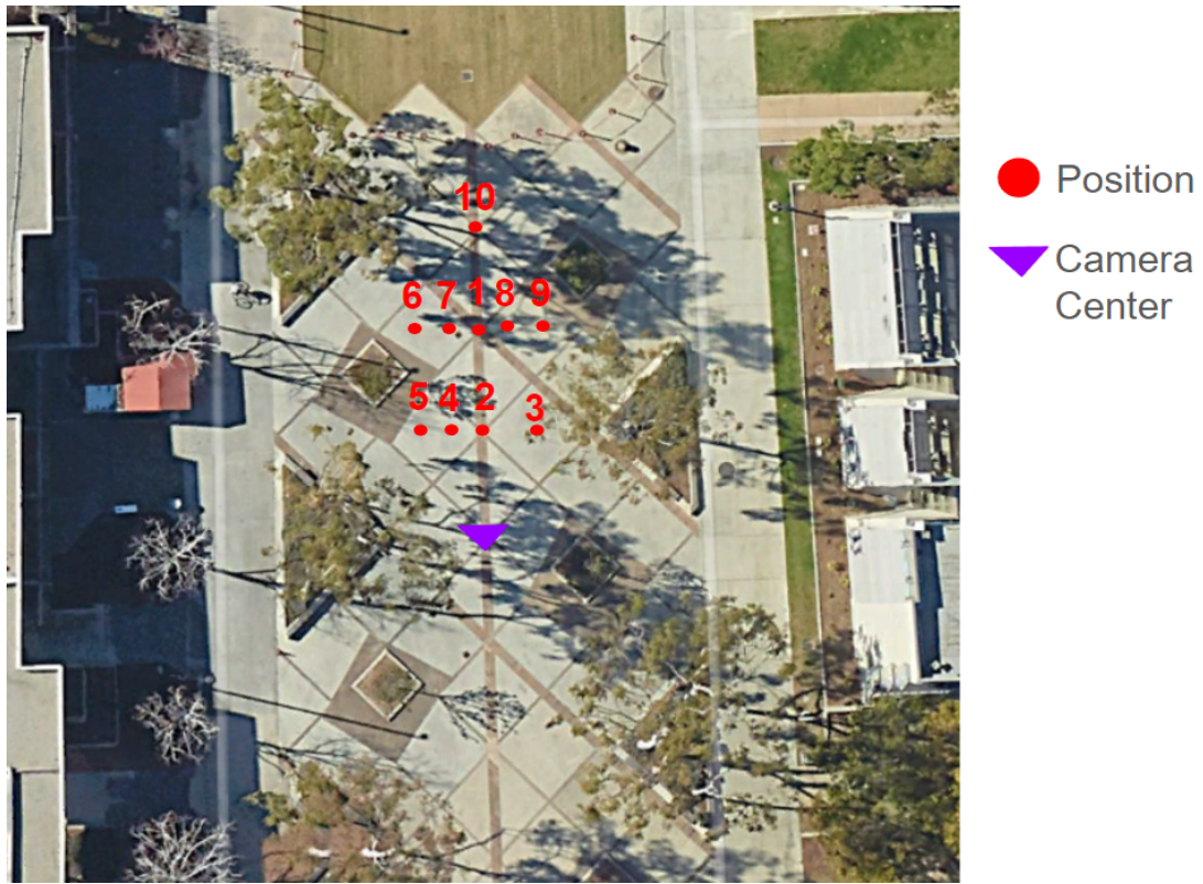
Figure 4.1. Experiment of testing the accuracy of IMU sensor absolute orientation readings and camera calibration parameters. Held a calibration board at each of 10 positions (Red Circles) while keeping camera still (Purple Triangle).
