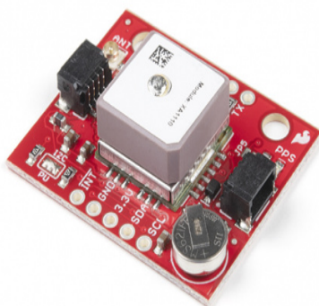
Figure 2.11. Image of SparkFun Quiic GPS Breakout Lite. Taken from Sparkfun website
