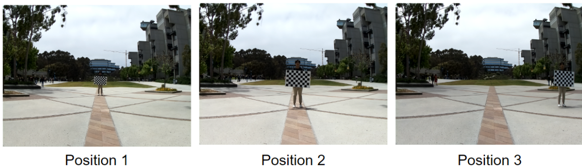
Figure 4.2. First 3 checkerboard positions to evaluate stereo camera calibration parameters and IMU orientation readings.
