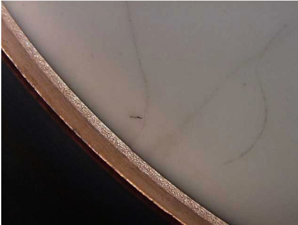
Figure 20. Crack at edge of ceramic after first braze test.
