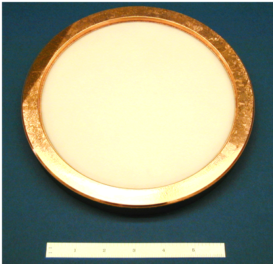
Figure 23. Window #2 as brazed.
