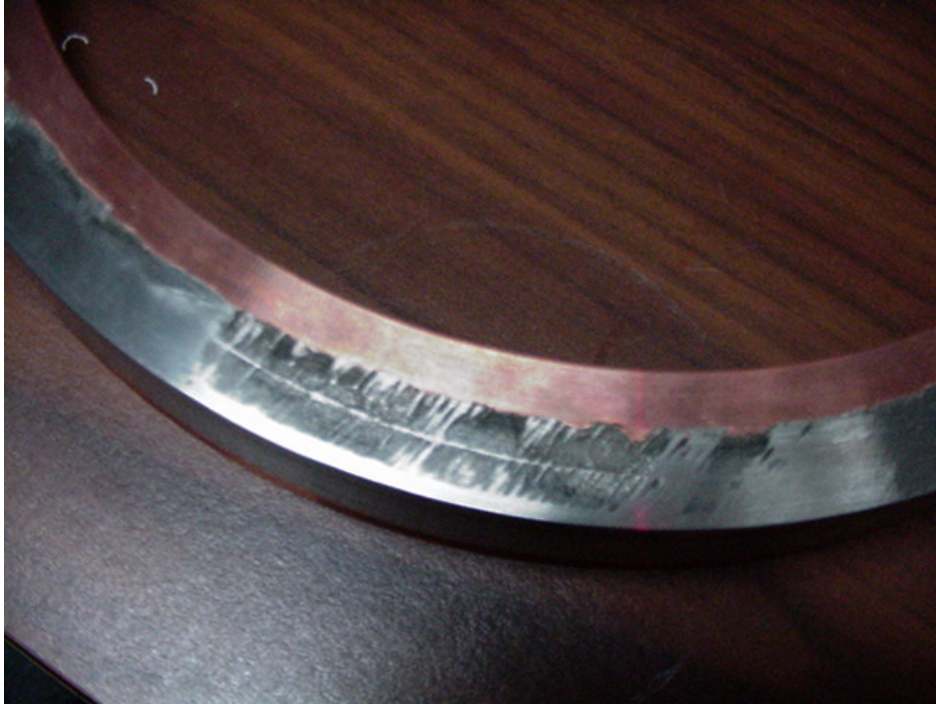
Figure 27. Etching damage on the stainless steel ring.
