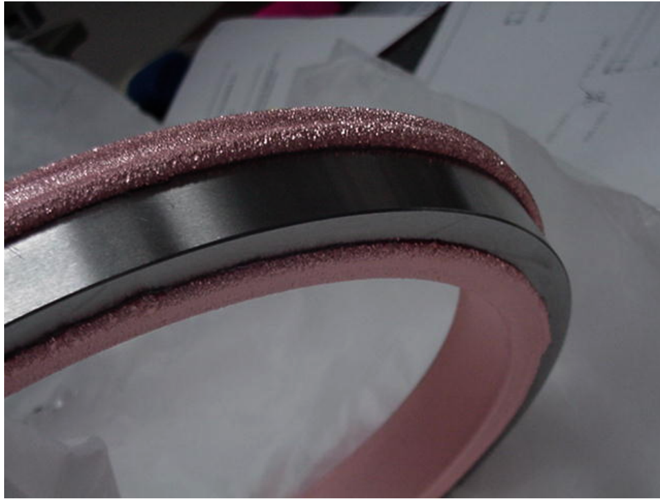
Figure 26. Copper build-up on the corner of the cooling ring.
