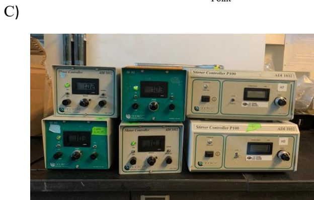
Figure 2.1. A) Comprehensive image of experimental set-up. B) Diagram of bioreactor vessel and notable parts. C) Applikon Motor Controller ADI 1012 & ADI 1032 boxes. D) Applikon P100 mixer motor attachment for bioreactors.
