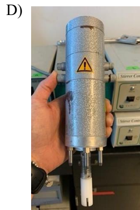
Figure 2.1. A) Comprehensive image of experimental set-up. B) Diagram of bioreactor vessel and notable parts. C) Applikon Motor Controller ADI 1012 & ADI 1032 boxes. D) Applikon P100 mixer motor attachment for bioreactors.
