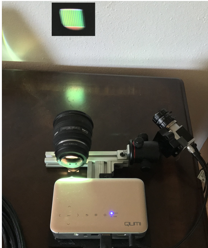
Figure 3: 2 combined photographs of prototype DFP system. Illumination is shown by splicing a second image with shorter exposure to illustrate projected pattern.
