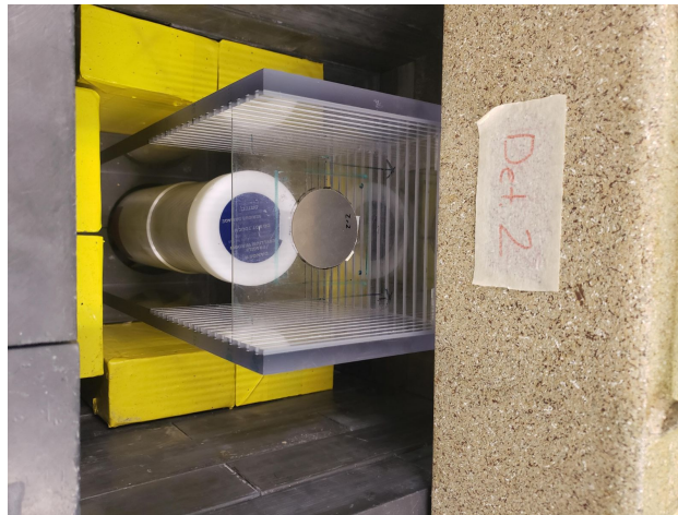
Figure 3.7: Picture of the HPGe detector setup used to measure gamma rays from in-beam activated foils. The detector is in a vertical configuration with a plastic shelving unit on top. In this picture, a zirconium foil is on the shelf. The detector is inside a lead box with a lead lid that can be rolled closed or open.
