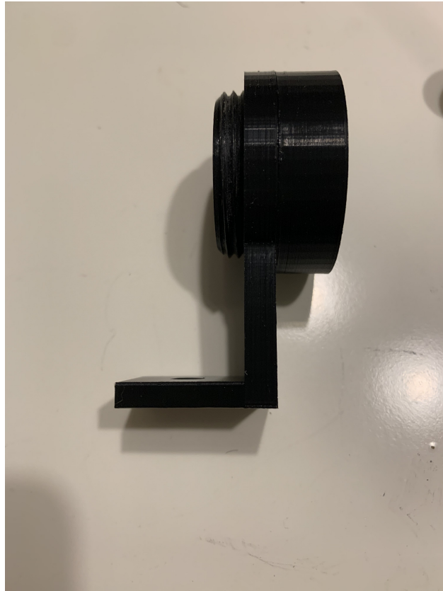
Figure 3.4: 3D printed holder and joint combined. This is used to attach the PMT and scintillator to the structural frame of STOF. PLA is used as the printing material.
