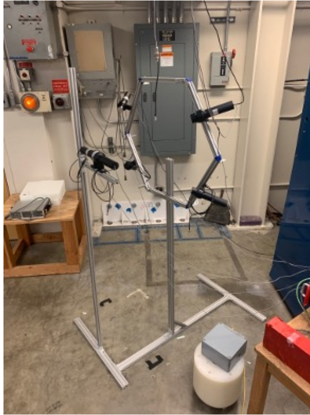
Figure 3.5: The STOF array consists of one target cell and four scatter cells arranged approximately 45 degrees from the beamline.
