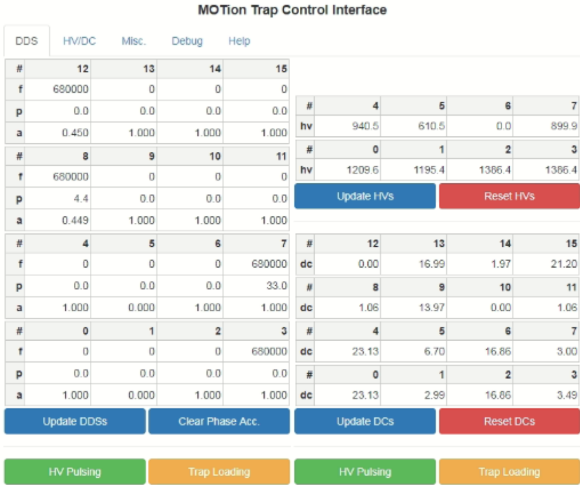
Figure 2.10: MOTion electronics control interface. A screenshot of the interface for the micro-controllers used to control the LPT rf, dc, and HV pulses and their timings is shown.
