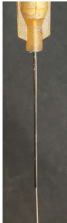
Figure 8: Liquid metal extruded as stream using high flowrate 2.3 ml/s.
