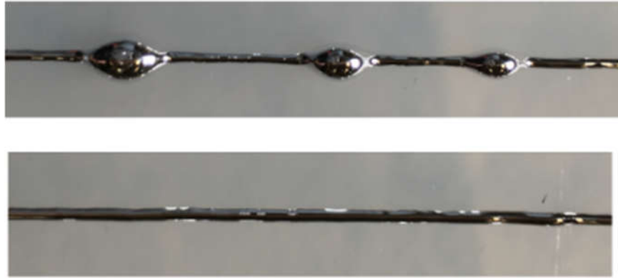
Figure 14: Top: trace with high variance using high-flowrate method. This occurs when extra liquid metal is printed. Bottom: trace with low variance using high-flowrate method when proper amount of liquid metal is printed.
