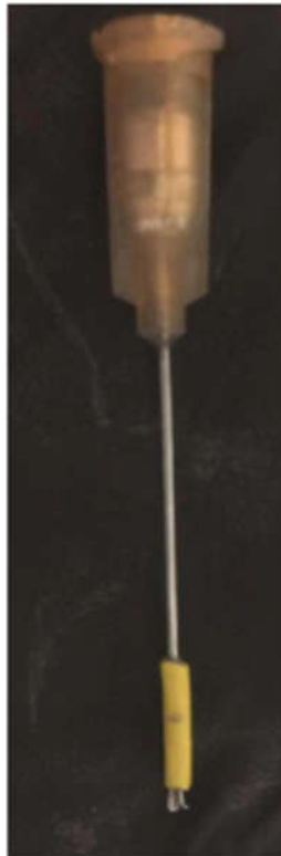
Figure 9: Stranded wire bristle attached at the tip of the needle.
