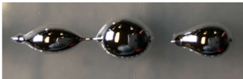
Figure 15: Failed printing with high-flowrate method using SOD larger than 0.3 mm, velocity around 10 mm/s and low flowrate.
