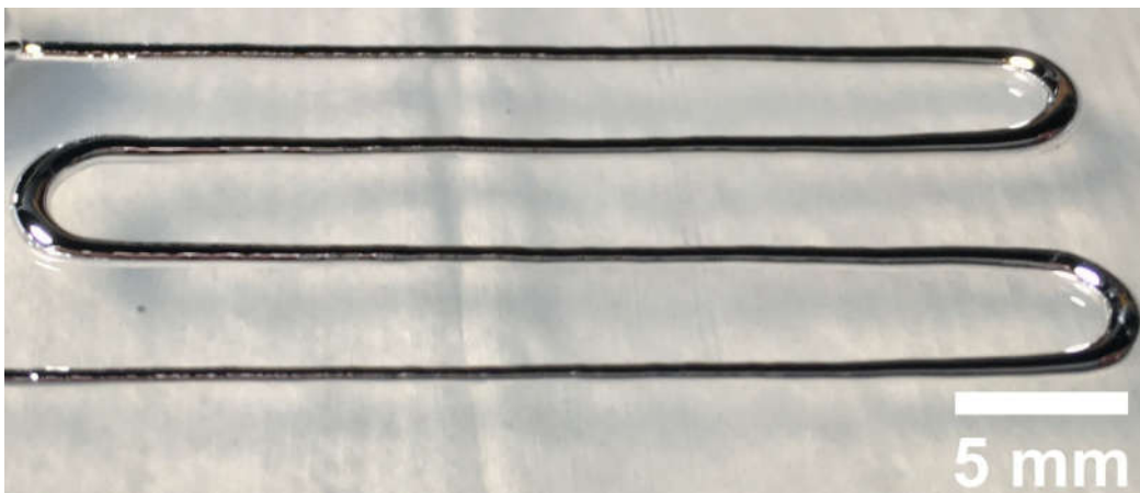
Figure 4: Bird's-eye view of printed liquid metal strain pattern using bristle method.
