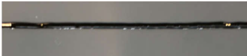
Figure 17: Trace with low variance printed by bristle method.
