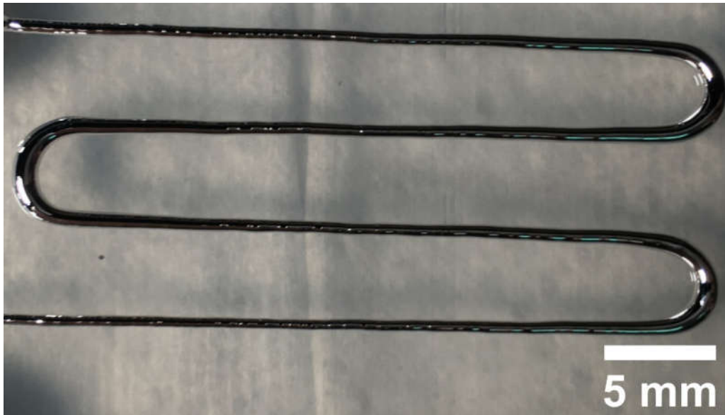
Figure 3: Top view of printed liquid metal strain pattern using bristle method.
