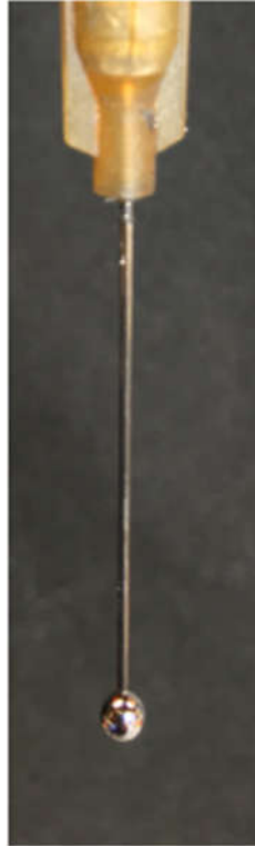
Figure 7: Liquid metal extruded as droplets using low flowrate 0.68 ml/s.
