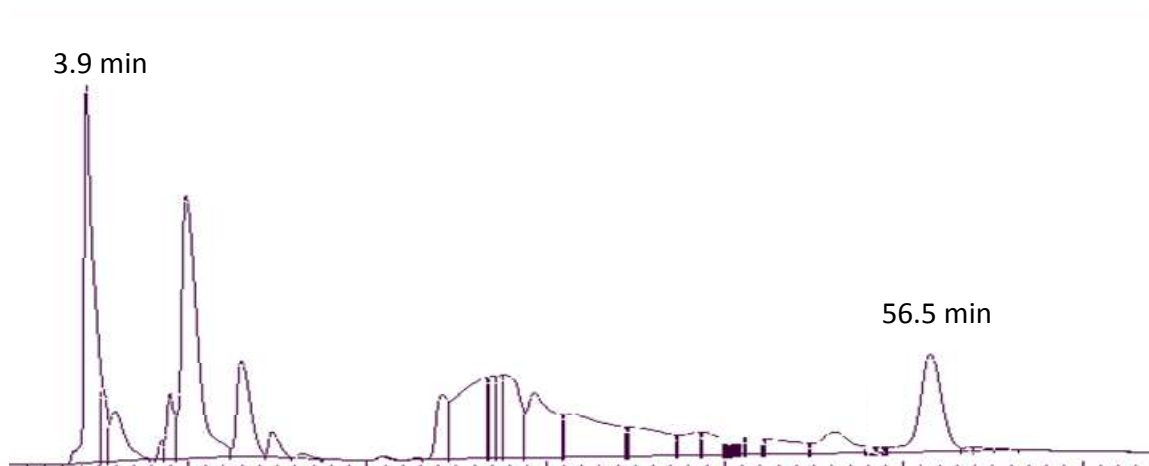
Figure 3.2 HPLC trace of isolation of labeled 5-forC and 5-carC from the mixture of MQ-sensitized photoreaction of ^{13}\text{C}_5 -5-methylcytidine. The fractions at retention times of 3.9 min and 56.5 are labeled 5-forC and 5-carC, respectively.
