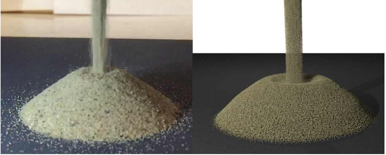
Figure 2.17: Avalanching. Sand is poured from a spout into a pile in a lab (left) and with our method (right). Our simulation is able to capture avalanching phenomenon.
