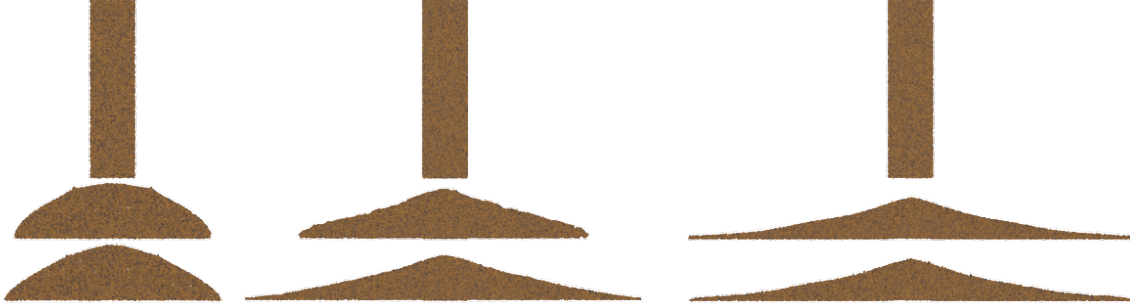
Figure 2.24: Fully implicit unilateral. Comparison of increasingly implicit time stepping schemes for 2D sand column collapse. The simulations on the left and at the center are run with the semi-implicit scheme with the regular and unilateral energy density functions respectively. The right-most figure shows a fully implicit scheme with our modified energy density function. Note that the unilateral density function with semi-implicit time stepping yields a good approximation of the fully implicit result, while the regular energy density suffers from artificial cohesion.
