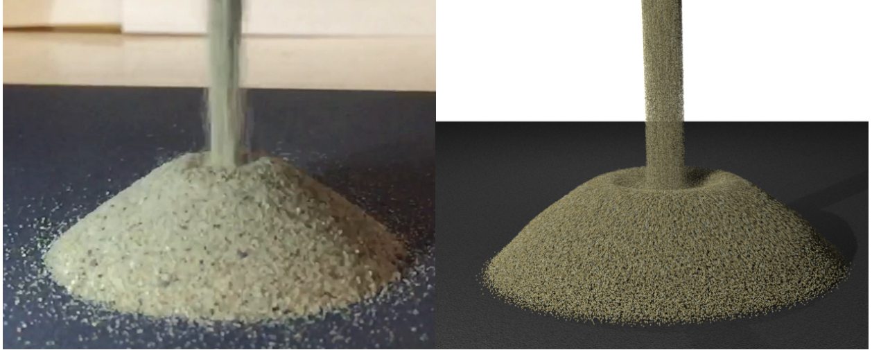
Figure 2.5: Avalanching. Sand is poured from a spout into a pile in a lab (left) and with our method (right). Our simulation is able to capture avalanching phenomenon.
