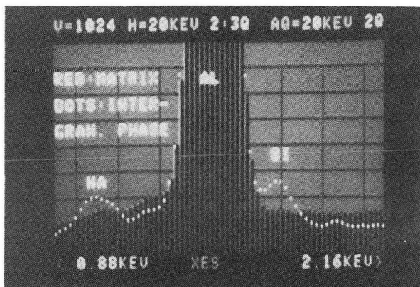
Figure 49. (a) Electron micrograph of a thick foil from the degraded region of an electrolyte subjected to 332 \text{ A hr/cm}^2 of charge transfer. The arrow indicates where sodium metal appears to have deposited. (b) Scanning transmission electron microscope identification of the sodium metal. Silicon appears to be associated with this particular sodium deposit as well.
