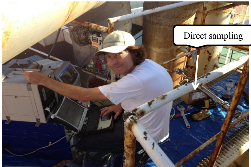
Figure 3-3.2 Measurement layout on auxiliary engine exhaust
