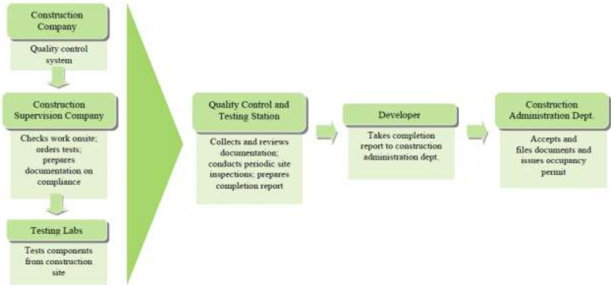
Figure 6-14. Roles and Responsibilities in Code Implementation and Enforcement in the Construction Process
