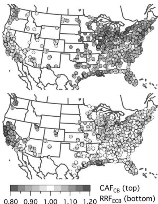
Figure 8. Climate adjustment factor ( CAF_{CB} ) for the A1B_US_M case (top), and the associated climate adjusted RRF ( RRF_{ECB} ; bottom). A CAF is calculated for all sites, but not all sites have an RRF (color figure available online).
