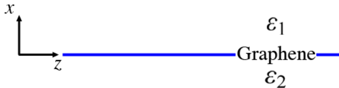
Figure 2.1 The monolayer graphene structure which can support SPP modes.
