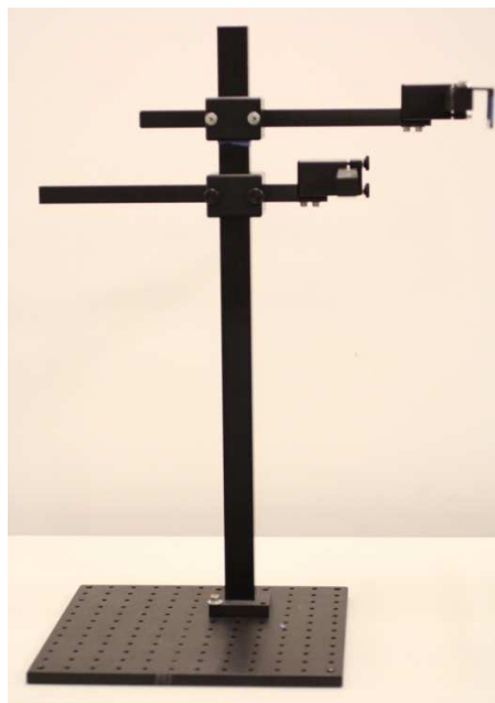
Fig 7.23: Visible picture of the camera mount used to hold the digital camera during the experiment
