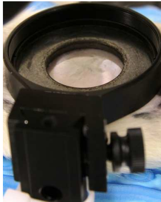
Fig 7.4 Mylar window placed flush against the animal's abdomen
