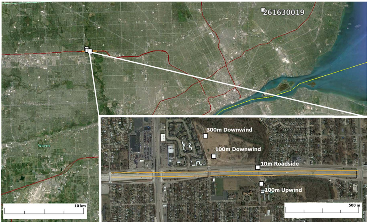
Fig. 1. The zoomed-in domain shows small white squares indicating the four monitoring sites at 10 m, 100 m and 300 m north of I-96 around the Eliza Howell Park and another site 100 m south of I-96. The yellow lines show the representative road links created to model the I-96 roadway segments. The expanded domain shows red lines segments from primary roads as described by the U.S. Census Bureau’s Topologically Integrated Geographic Encoding and Referencing (TIGER) road data. The AQS site E 7 Mile Road (26-163-0019) used as representative urban background site is also shown by a small white square. (For interpretation of the references to colour in this figure legend, the reader is referred to the web version of this article.)
