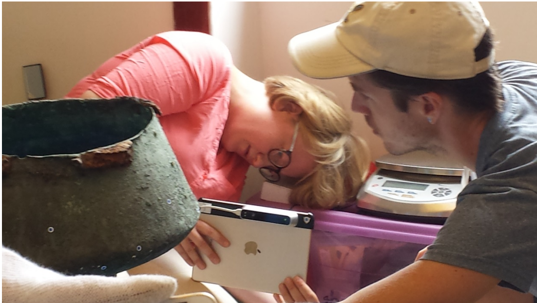
Figure 4. Sara Eriksson and Aaron Brown capturing data for 3D model of bronze casserole using Structure Scanner mounted on iPad.
