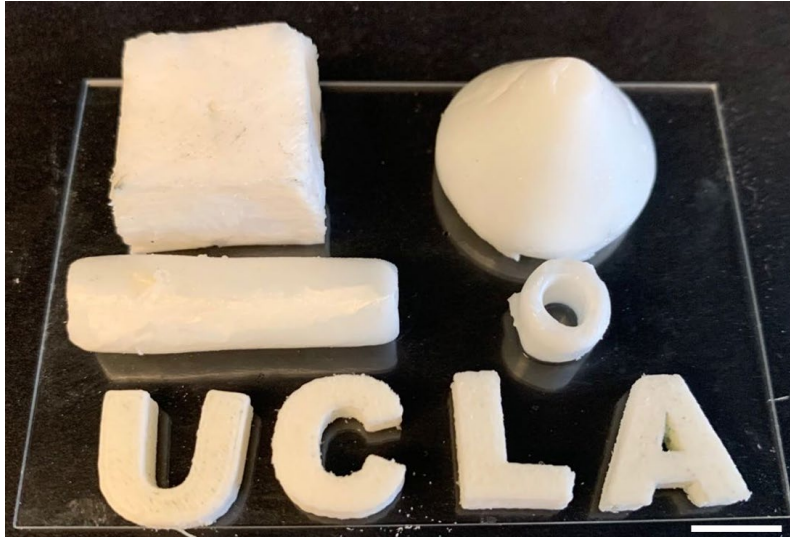
Figure 2.2 PVA hydrogels with different shapes obtained with freeze-soak method. Scale bar = 1 cm.
