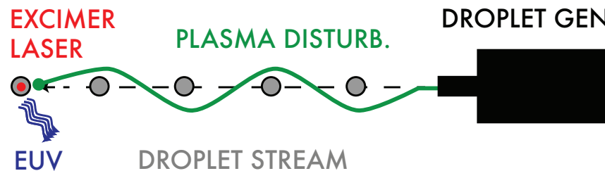
Figure 1.1: A simplified figure of the EUV generation process. Liquid tin is ejected from the generator and ionized by the excimer laser, releasing a photon of EUV light. The resulting tin plasma byproduct (free-electron diffusion, ion-acoustic waves, thermofluidic, and electromagnetic effects) disturbs the transverse displacement of droplets upstream.
