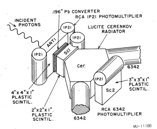
Fig. 3. Gamma-counter telescope.
