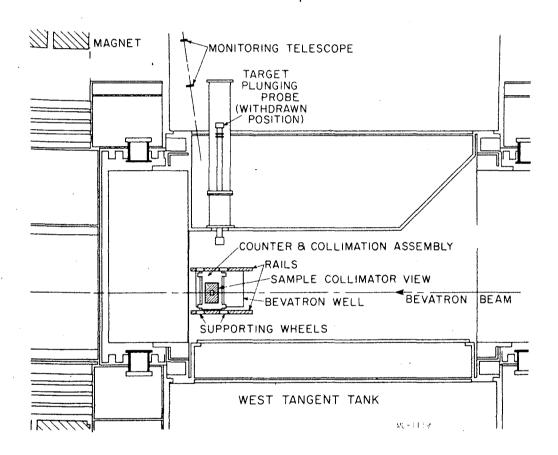
Fig. 2. Experimental layout at Bevatron.
