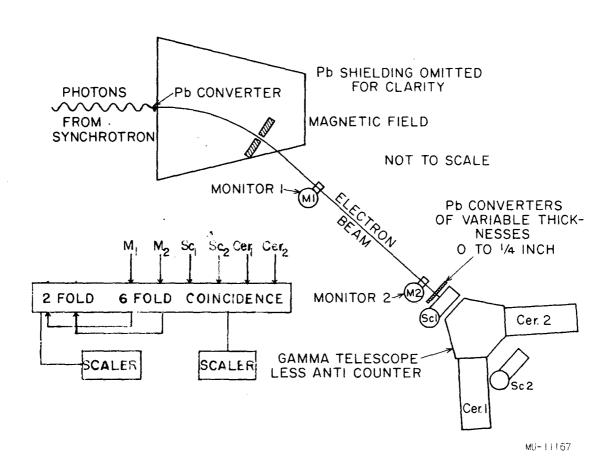
Fig. 7. Gamma-counter telescope calibration layout.
