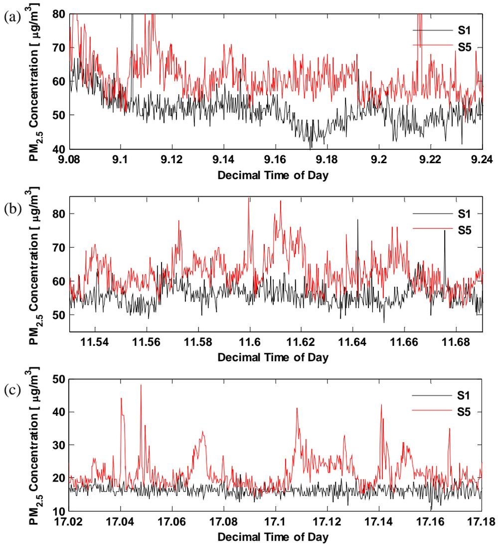
**Figure 4.** Time series (~ 10 minutes) of PM<sub>2.5</sub> concentration at site1 (windward side) and site 5 (leeward side) in Los Angeles during (a) morning, (b) noon and (c) afternoon. (Note: data are collected on 06/19/2008 in (a) and (b), 06/30/2008 in (c).)
