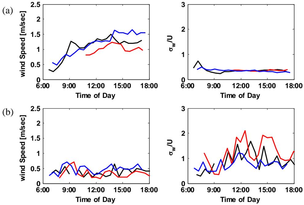
**Figure 1.** Mean wind speed and vertical velocity fluctuations in (a) Huntington Beach and (b) Los Angeles. (Note: black, red and blue indicate three different days.)
