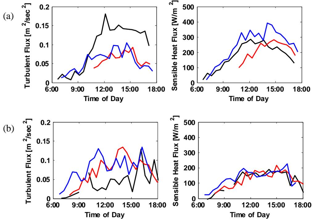
**Figure 2.** Turbulent flux and sensible heat flux in (a) Huntington Beach and (b) Los Angeles. (Note: black, red and blue indicate three different days.)
