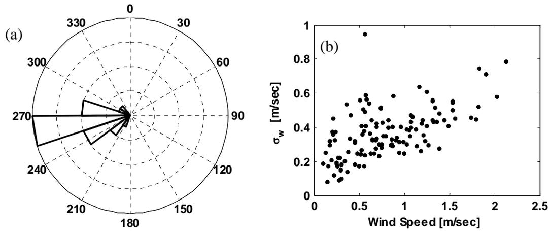
Figure 5. (a) Wind rose and (b) relation between wind speed and  $w_{rms}$  on 07/02/2008 at Long Beach.
