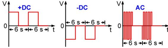
Fig. 3. Actuation signals for electrowetting testing.
