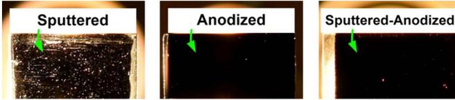
Fig. 2. Results of pinhole test for the three types of  $\text{Ta}_2\text{O}_5$  films.
