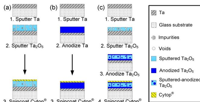
Fig. 1. Process flow to prepare (a) sputtered, (b) anodized, and (c) sputtered–anodized Ta<sub>2</sub>O<sub>5</sub> EWOD devices.
