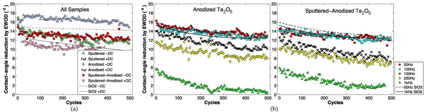
Fig. 4. Electrowetting-induced contact-angle reduction measured on EWOD devices under (a) dc actuation and (b) ac actuation. The performance of thermal SiO<sub>2</sub> [10] is included as a high-standard reference after an exponential curve fitting of the experimental data.
