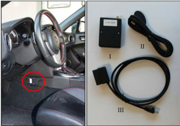
Figure 1. (Left) On-board data logging device connected to the vehicle. (Right) I. the device II. Antenna III. OBD-II connector cable.
