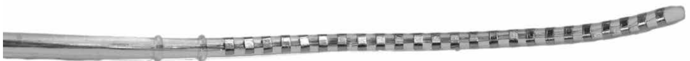
Figure 2. The standard Nurotron electrode array. The electrode holds 24 Pt90Ir10 foil contacts in an elastomer carrier. The round window marker is shown as the ring on the left. The mean insertion depth for the array was 426° (n=60, initial Nurotron clinical trial data).
