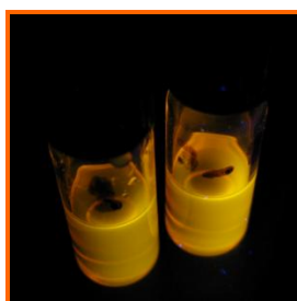
Figure 3.22 No change in fluorescence is observed for CdSe QDs (5 \mu\text{M} ) before (left vial) and after (right vial) the addition of alkoxyamine 3.20 (1000:1 moles of alkoxyamine 3.20 :QD) in toluene solution.
