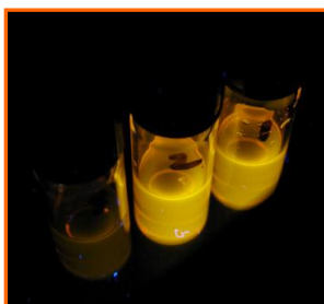
Figure 3.14 Fluorescence of 5 \mu\text{M} CdSe QDs in toluene in the presence of (from left to right): carboxylic acid nitroxide 3.10 (2500:1 moles of nitroxide 3.10 :QDs), TEMPO (2500:1 moles of TEMPO:QDs), and no additive upon illumination with a TLC lamp at 366 nm
