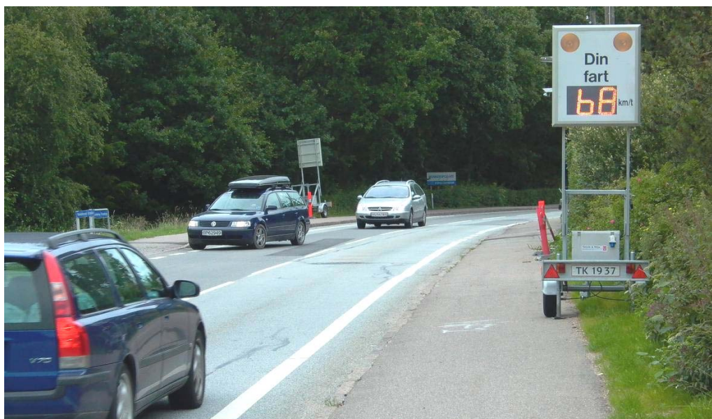
Figure 6.11. Speed monitoring is normally used as a measure to improve traffic safety. If it has an effect on reducing the actual speed it can also have a noise reducing effect [10].
