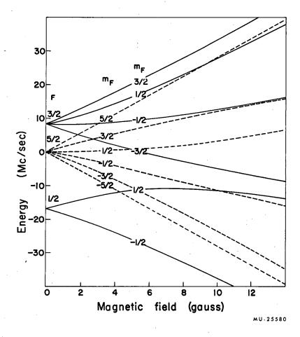
Fig. 2. Breit-Rabi diagram for the  $^2P_{3/2}$  electronic state of Ga  $^{68}$  (calculated for a = +1.660 Mc/sec, b = -10.276 Mc/sec).
