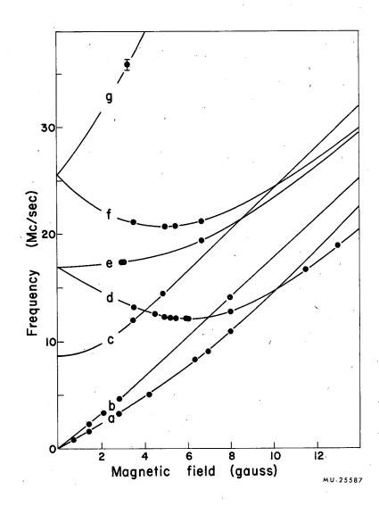
Fig. 9. Comparison with the  $^2P_{3/2}$  observed resonances to the theoretical transition frequencies calculated for a = +1.660 Mc/sec, b = -10.276 Mc/sec. Resonance identifications are listed in Table IV.
