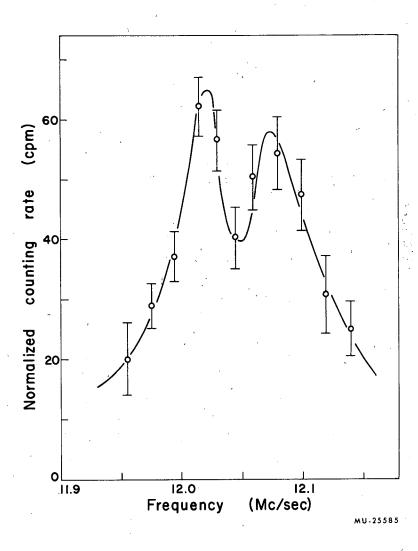
Fig. 7. A resonance corresponding to the  $(5/2, 1/2) \longleftrightarrow (1/2, 1/2)$  transition in the  $^2\mathrm{P}_{3/2}$  electronic state of Ga $^{68}$ . (H = 5.994 gauss).
