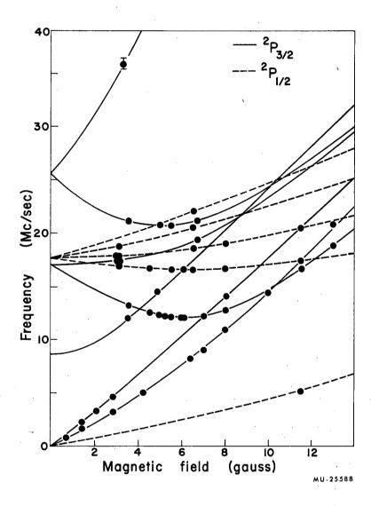
Fig. 10. Comparison with the observed resonances to the theoretical transition frequencies calculated for a = + 1.660 Mc/sec, b = - 10.276 Mc/sec, and  $\Delta \nu$  = + 17.574 Mc/sec. The solid lines represent the  $^2P_{3/2}$  electronic state, and the dashed lines the  $^2P_{1/2}$  state.
