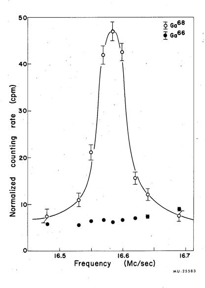
Fig. 5. A resonance corresponding to the transition  $(3/2,-1/2)\longleftrightarrow (1/2,-1/2)$  in the  $^2P_{1/2}$  electronic state of Ga $^{68}$ . (H = 5.491 gauss.) The Ga $^{66}$  background component is also displayed.
