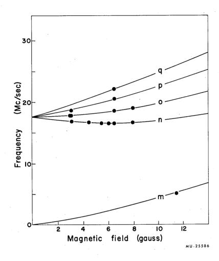
Fig. 8. Comparison with the  $^2P_{1/2}$  observed resonances to the theoretical transition frequencies calculated for  $\Delta \nu = + 17.574$  Mc/sec. Resonance identifications are listed in Table IV.
