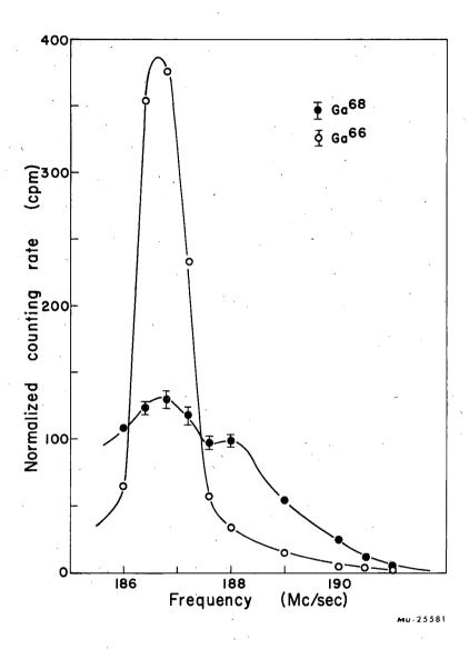
Fig. 3. Ga<sup>66</sup> and Ga<sup>68</sup> resonances observed at H = 99.965 gauss.
