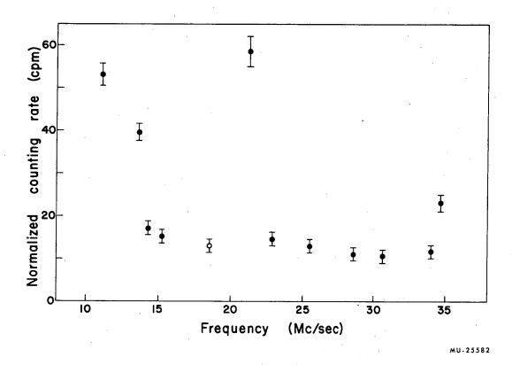
Fig. 4. A search for possible resonances, conducted at 3.020 gauss. (The open circle point displayed at 18.5 Mc/sec was taken with the rf off.)
