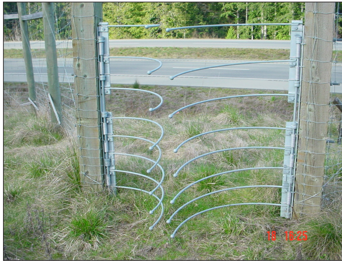
Figure 2. One-way gate designed for moose and deer.
