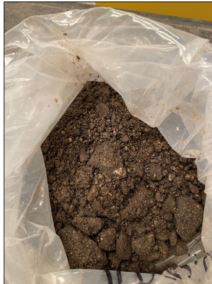
Figure 2.9: GLE-162: Unbound asphalt-treated base material.
