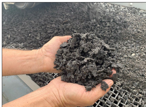
Figure 4.9: SBD-2: Asphalt rubber chip seal millings on multi-unit train screen.
