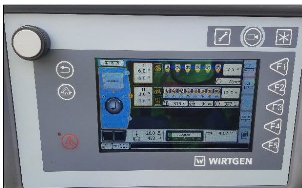
Figure 3.21: SB-135: 08/23/21 - single-unit train foamed asphalt at 20 fpm.
