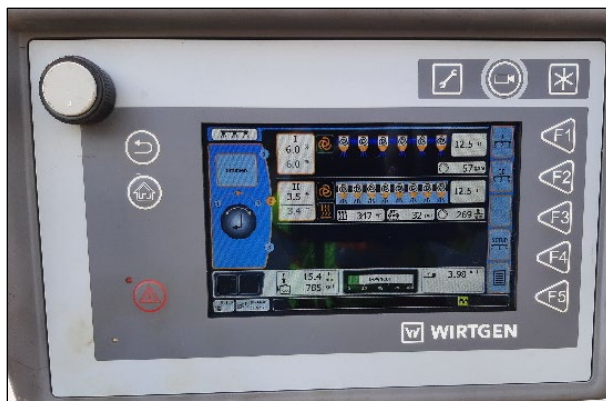
Figure 3.19: SB-135: 08/23/21 - single-unit train foamed asphalt at 15 fpm.
