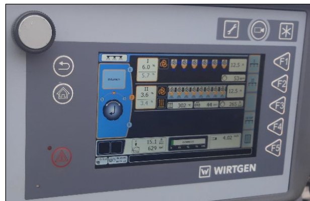
Figure 3.20: SB-135: 08/24/21 - single-unit train foamed asphalt at 15 fpm.
