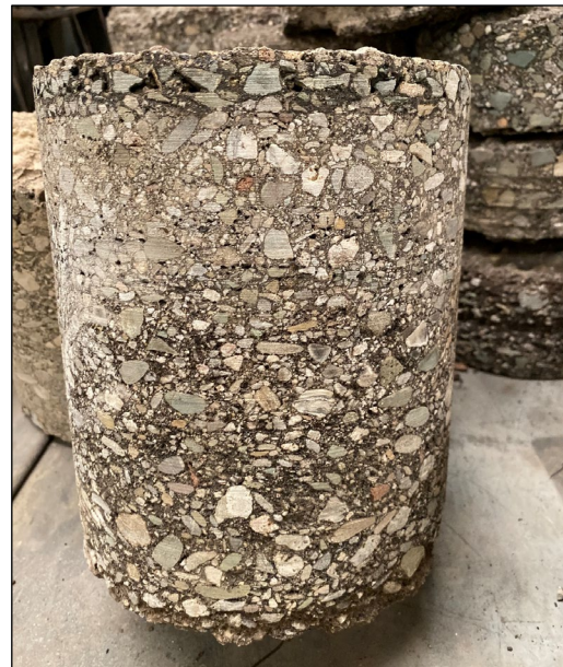
Figure 2.7: GLE-162: Core from thicker section with multiple asphalt concrete layers.
