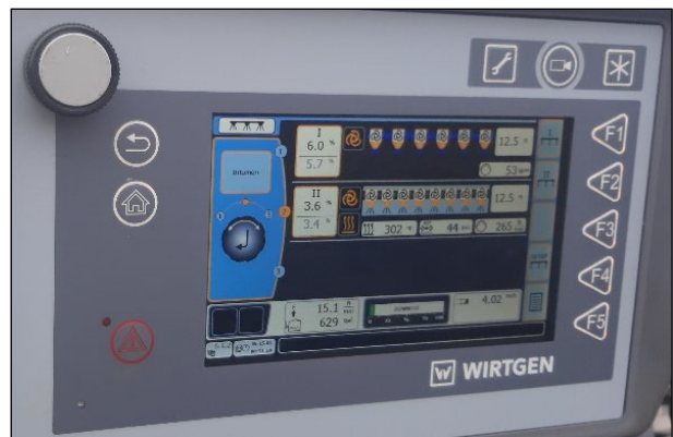
Figure 3.20: SB-135: 08/24/21 - single-unit train foamed asphalt at 15 fpm.
