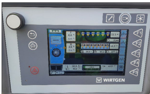
Figure 3.21: SB-135: 08/23/21 - single-unit train foamed asphalt at 20 fpm.
