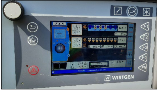
Figure 3.23: SB-135: 08/25/21 - single-unit emulsified asphalt at 20 fpm - start of section.
