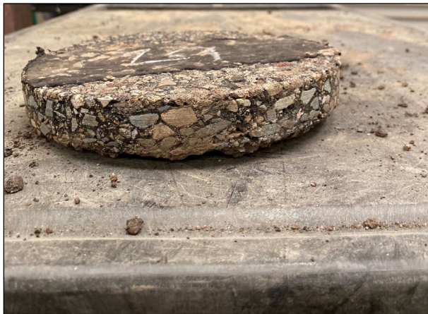
Figure 2.6: GLE-162: Core from RHMA-G overlay.
