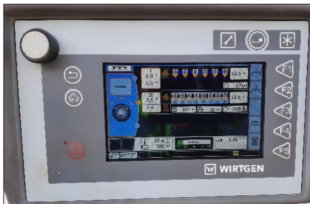
Figure 3.19: SB-135: 08/23/21 - single-unit train foamed asphalt at 15 fpm.
