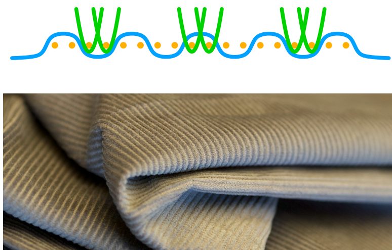
Figure 2.10: Corduroy. Top: Side-view of weave structure. Bottom: Photograph of corduroy fabric.
