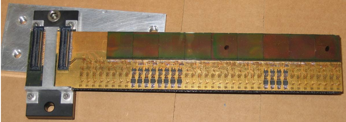
Figure 46: A prototype ladder showing low mass PCB, MIMOSA5 detectors and driver electronics bonded to a mechanical carbon fiber and reticulated vitreous carbon foam based carrier.
