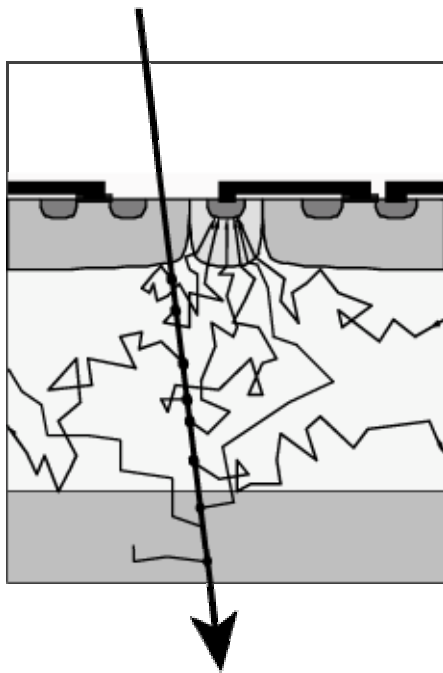
Figure 34: Epitaxial Silicon used as a sensor. In this design, a primary ionizing particle creates free charges in the epitaxially grown Si layer that is a few tens of microns thick and a few electrons in the bulk layers. The liberated charges are then free to diffuse towards a potential well structure at the top of the sensor where they are extracted and readout into a DAQ system.
