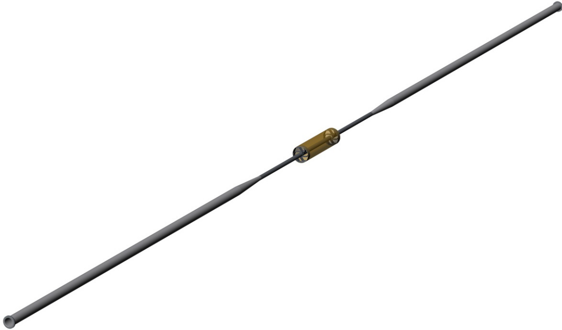
Figure 61: Beam pipe structure with outer support barrel in the center.
