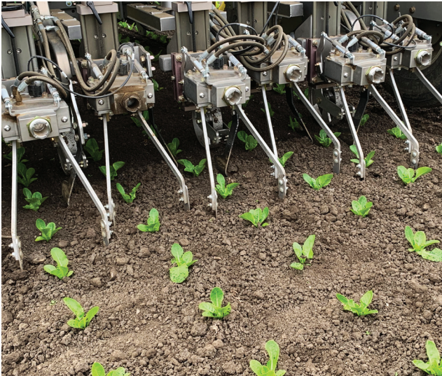
Figure 8. Automated weeder using a split knife that opens around the lettuce plant and closes between lettuce plants to remove weeds in the seedline.
