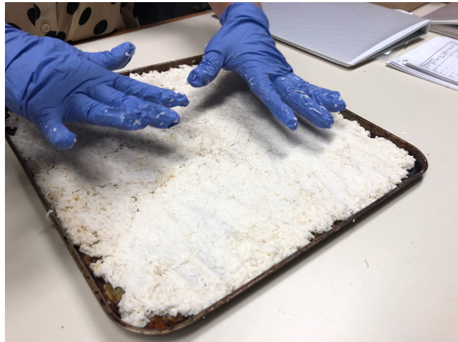
Figure 2: Manioc after being grated and expelled of water, before being placed in desiccator.
