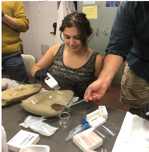
Figure 5: Using sonicating facial spatula in a circular motion and extracting the material with pipette.
