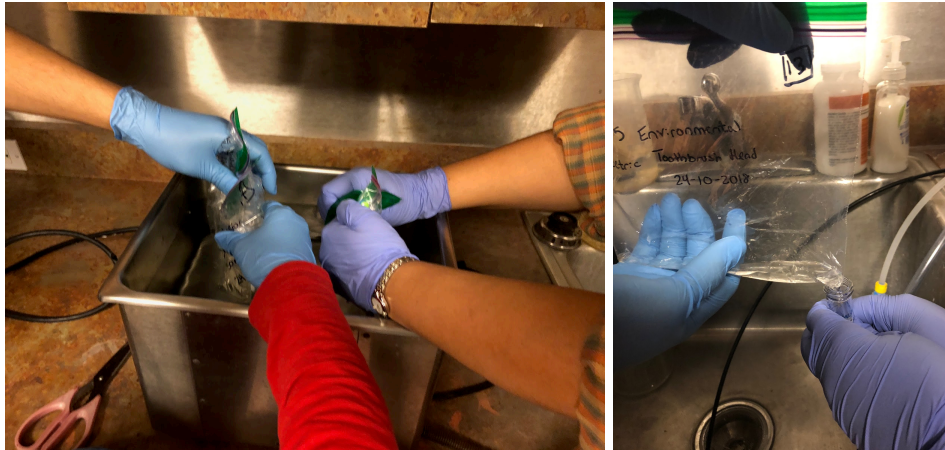
Figure 6: A. Holding scrubbing instruments in sonic bath (left). B. Cutting bottom corner to carefully pour contents into test tube.
