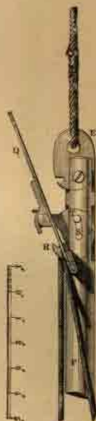
FIG. 40.—Instrument for slipping the Cylinder at intermediate depths.
