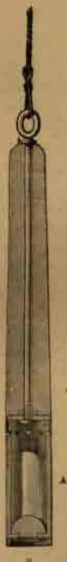
FIG. 18.—The Valve Sounding Lead.
