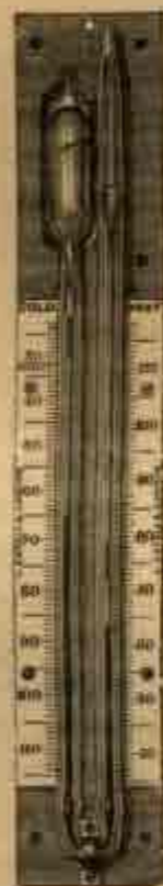
FIG. 27.—Six's Deep-Sea Thermometer.
